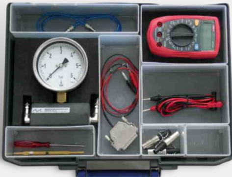
**Calibration kit** for calibrating pressure and temperature.
